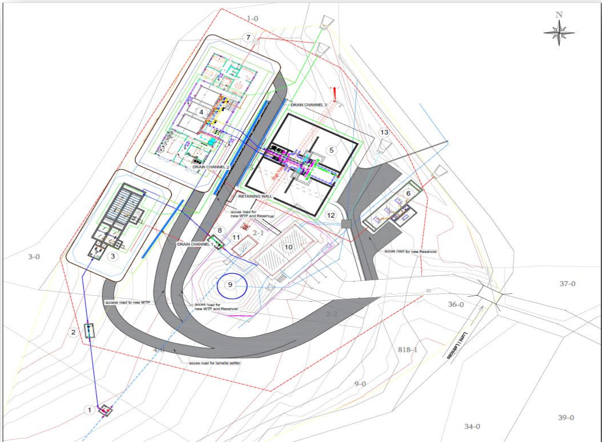
Figure 7. General layout of the existing and newly planned WTP with appurtenant structures-orthophoto map 1: 500
